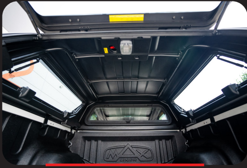
Internal steel structure for increased roof carry capacity*
