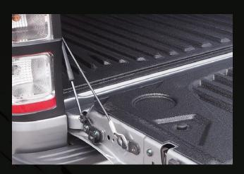
Maxliner bring comfort to your truck bed. Tail gate lift assist enable easy and convenient access to your vehicle truck bed.
